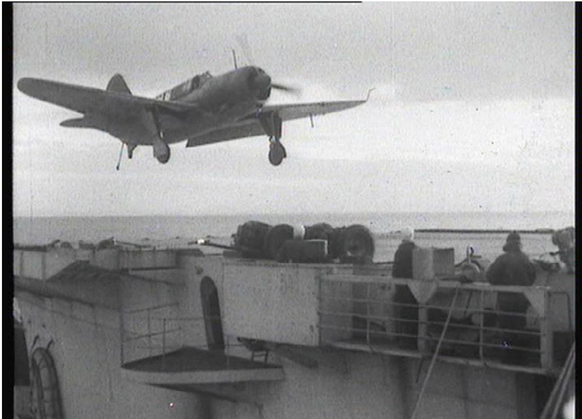
Figure 2 - Arrestor hook landing on a carrier
